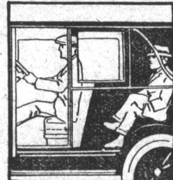
Note also that front seat adjusts backward to make tall people comfortable without crowding people in rear seat.
