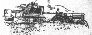
The McCormick-Deering Harvester-Thresher saves 20 cents per bushel over old methods in the harvesting of grain. It requires 15-30 power.
