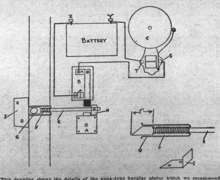
This drawing shows the details of the gong-type burglar alarm which we recommend that our subscribers install in their chicken coops to scare away thieves. We have explained in this article how to make the alarm and install it but if you do not want to bother with making one we can supply it complete for \$6.50, which is just what they cost us. You will need three dry cell Latteries to operate the alarm.
