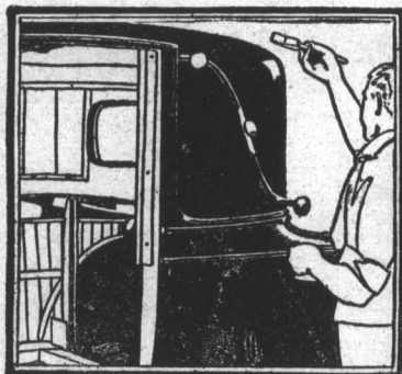
The clay model, when finished looks exactly the same as the finished body will look.
