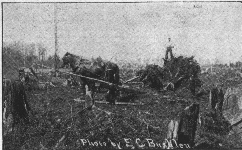
The Popular Capstan Type of Stump Puller at Work on a Large Stump.
