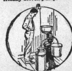
The constant speed of the electric motor means better separation of the cream.
