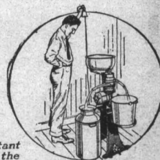
Running water upstairs and downstairs with an electrically driven pump.
