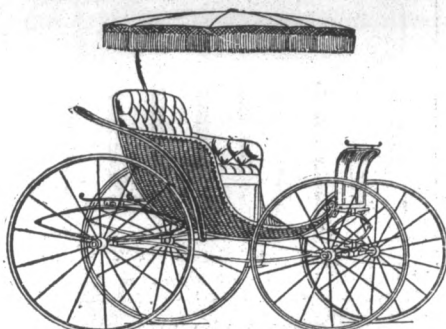
No. 277½—Pony Phaeton. Body constructed of finest imported German reed woven on hand forged wrought iron frame. Stylish, handsome, durable, and like the rest of our pony work, a job in which grown-ups as well as children can ride with comfort.
