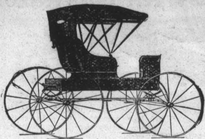
No. 149—New Autostyle Buggy. Twin Auto-Belgian type seat with large, round corners and beautiful curves. Handsome, stylish, comfortable. All wrought gear and best second growth hickory gear woods. Axles arch, high arch or very high arch as desired. Soft, easy-riding springs, oil tempered. 2,500-mile, long distance dust-proof axles. Our A-grade select hickory wheels and high bend select white hickory shafts with 36-inch leather tips. Latest auto design top with "automobile" leather. Painting and trimming optional.
