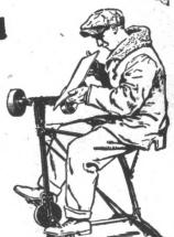
Pedals like a bicycle. pressure required—no water or oil to cool the steel. The head swivels, making the most awkward tool easy to grind.
