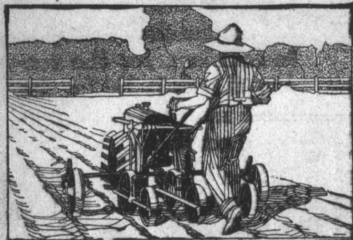
A Utilitor and three-row gang seeder will drill or hill 35 different kinds of seeds.
