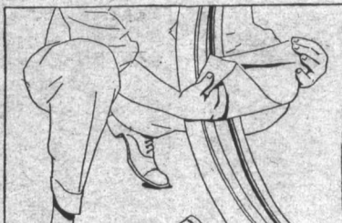
RIM-CUT PATCH BEING INSERTED
