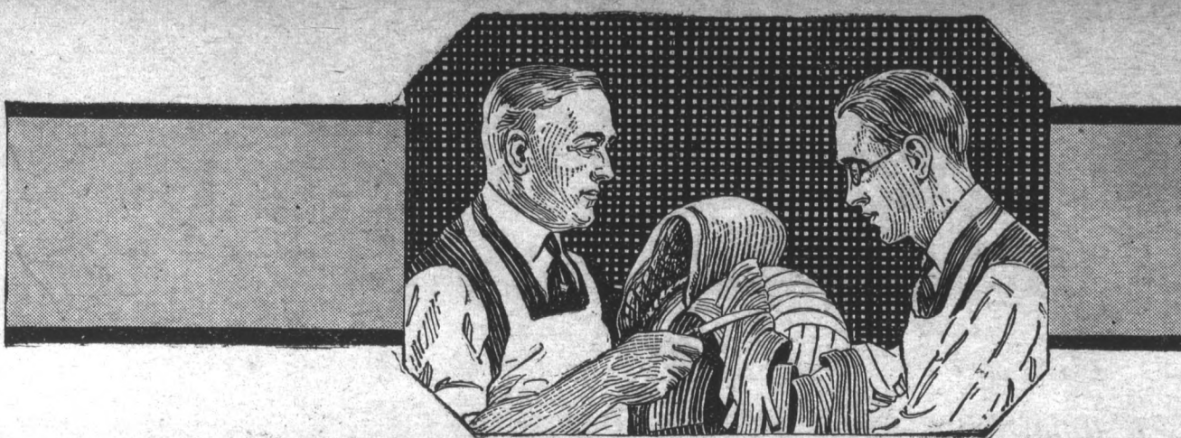
Examining the tire layers after 15,000 miles
