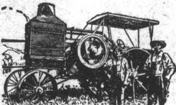
OilPull Number 174, built in 1909, 12 years ago. The owner C. J. Chandler, Lincoln, Kan., says it will last another decade. The only renewed parts of motor are four piston rings.
