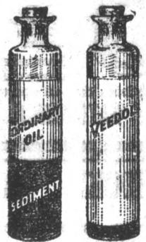
Showing sediment formed after 500 miles of running
