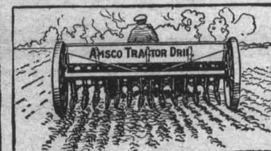
The Amsco Tractor Drill Tractors speed and accuracy utilized by the Fordson owner with the Amsco special drill. Force feed makes positive planting.
