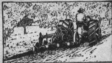
Special Oliver Orchard Plow Fordson orchard plowing is done thoroughly with the Oliver special orchard gang. Branches and trunks are not injured.
