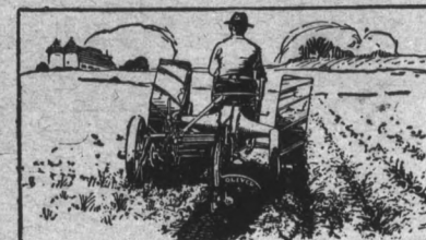
Oliver Single Bottom Sulky For deep mouldboard plowing in trashy conditions with the Fordson. Similar in construction to world famous No. 7 gang.
