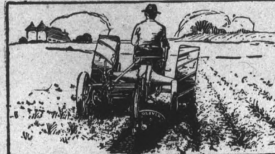
Oliver Single Bottom Sulky For deep mouldboard plowing in trashy conditions with the Fordson. Similar in construction to world famous No. 7 gang.
