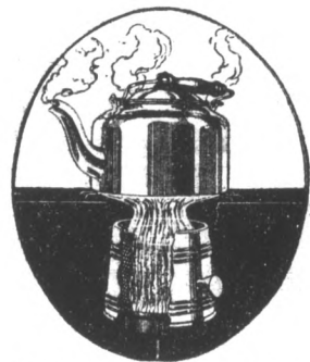
Cut-away view of the Florence burner, showing how the heat is focused right on the cooking vessel.
