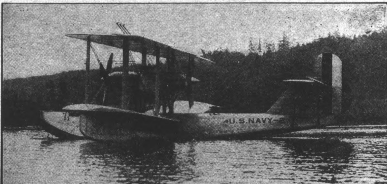
The Boeing BP-1 seaplane was built at Seattle for a non-stop flight to Honolulu. When this giant plane lifted its twelve tons of steel and wood, it represented a milestone in airplane building.
