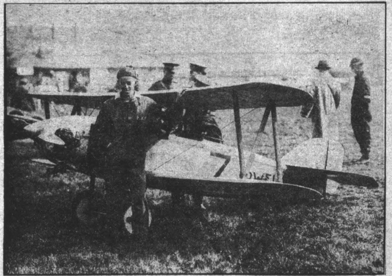
This was the smallest plane entered in the aviation meet at Mitchell Field, Long Island. It is a tiny Powell Racer with a 17.7 H. P. Bristol Cherub motor.
