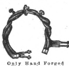
Only Hand Forged Wrought Iron would Stand being Hammered and Bent Cold like This.
