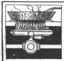
The intense heat of a gas stove burner is due to the flame striking and spreading under the entire base of cooking utensils.
