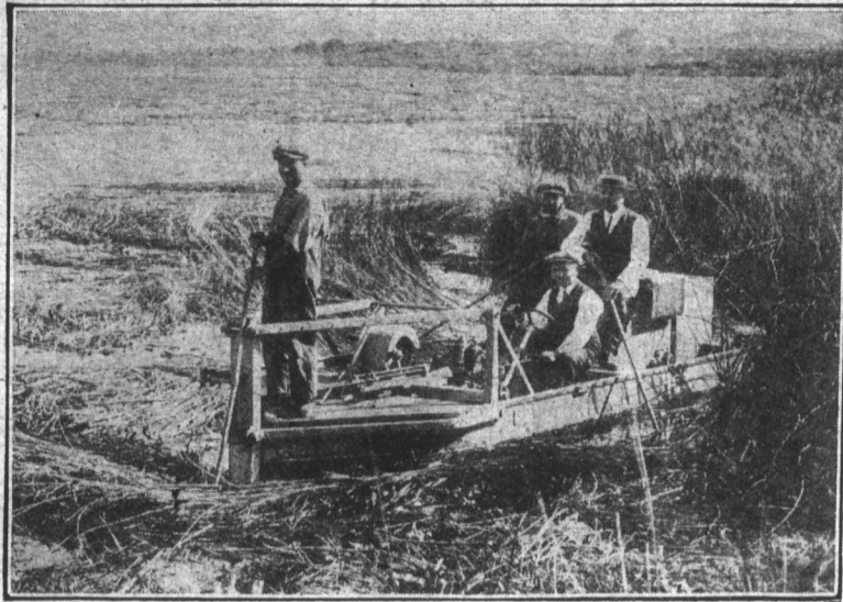
Mosquitoes have been exterminated and swamp land reclaimed by this aquatic harvesting machine for weeds, invented by a Frenchman. The boat travels on land as well as on water.
