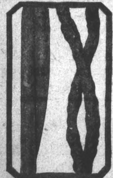
Leadclad left - Ordinary fence right. Photographed after 5 years service.
