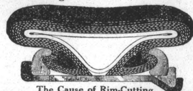
The Cause of Rim-Cutting
