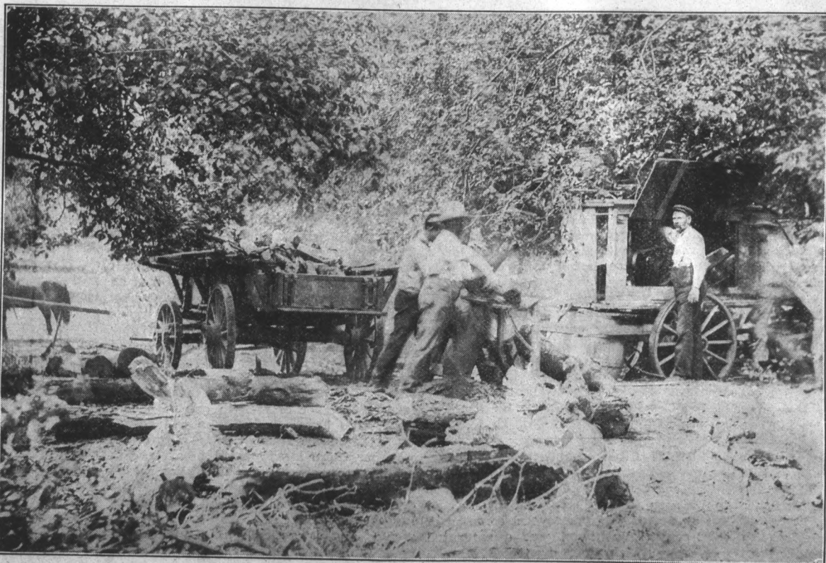
Utilizing the Sprayer Engine to Advantage in "Buzzing" Up the Stove Wood without Dismounting it from Rig.
