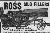
The Ross is the only machine of this type that is equipped with steel cutting apparatus, steel blower disc, and steel truck. Other machines of this type are furnished with cast iron cutting apparatus, cast iron blower disc. The steel equipment makes the Ross indestructible, and the most reliable and durable silo filling machines on the market. Strong claims made for strength, capacity, durability and ease in feeding. Ask for large catalog The E. W. Ross Co., Box 114 Springfield, Ohio
