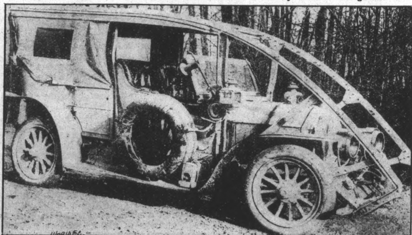
French Military Autos are Equipped with Steel Rails which Cut through Barbwire Entanglements.
