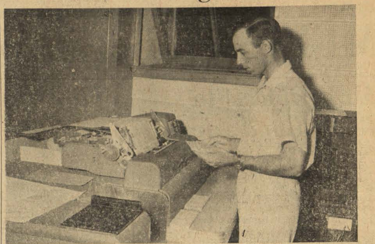
HERE'S THE WAY IBM machines work: The records are punched into cards that fit an International Business Machine tabulator as shown above. Cards that MSC Dairyman Alvin Thelen feeds the machine are tabulated on one sheet. The electrical calculator can quickly produce complete records from the cards on individual cows, herds and Associations.
