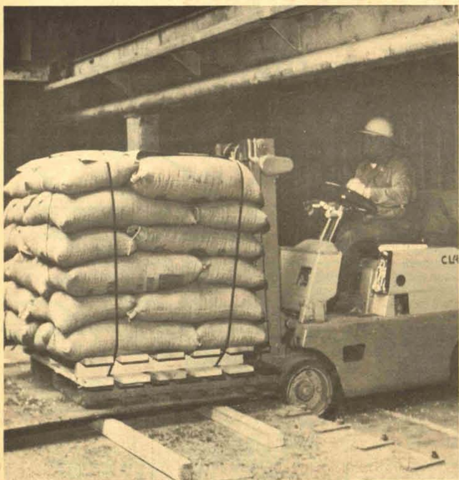
MECHANICAL POWER — largely replaces man-power in stowing beans into the ship's hold. Using the fork-lift, two men can stow the beans faster than was common with an 8 or 10-man crew. At the English port, they will unload in similar manner and with large savings in labor cost.
