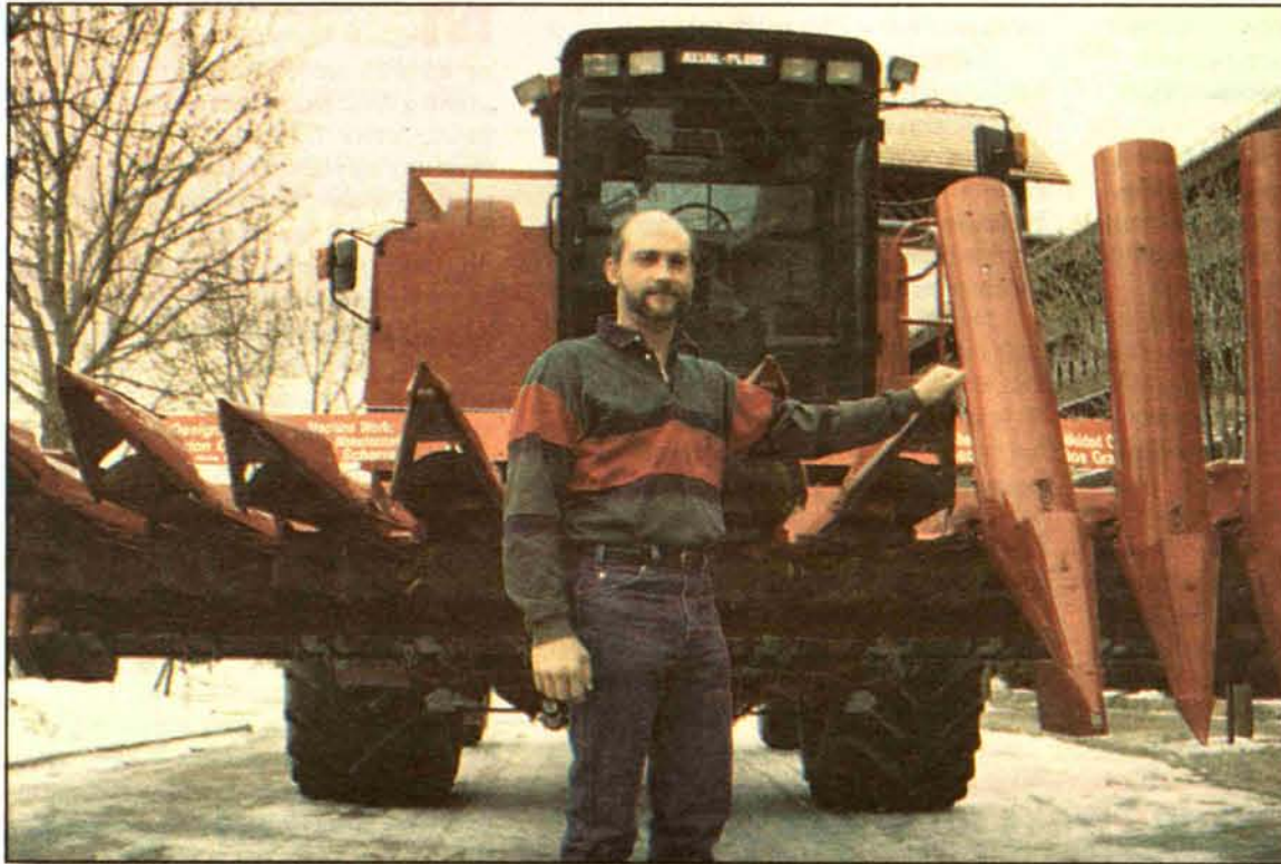
Making the decision to switch to 15-inch rows was easier than finding a corn head to harvest them with for Farm Bureau member Don Morse of Saginaw County. He used a design from a three-row prototype created by Illinois farmer Marion Calmer to build the first 11-row, 15-inch corn head in the country. Morse was pleased with how well the narrow-row head worked on harvesting over 400 acres of corn last year.
