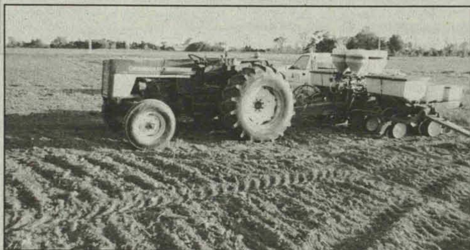
This planter provided by Alpine Fertilizer is equipped to make three different fertilizer treatments by a simple selector switch.
