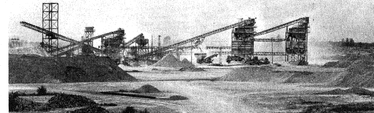
THIS IS THE SIXTH Quarry crusher now in use. The rest have been laid to rest. This plant is truck fed, says Dast.
