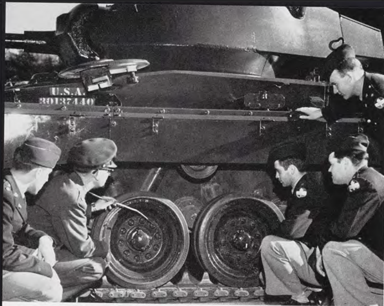
Major George Major explains the suspension system of an M-24 light tank to a group of Armor cadets, placing particular emphasis on the damage that a land mine could do to the tracks.
