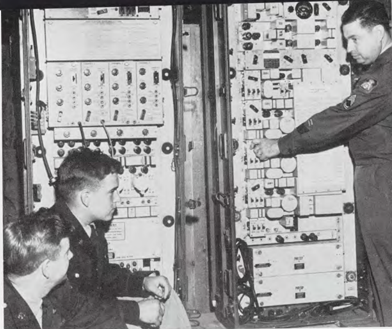
Sergeant First Class Charles Doering explains to cadets Dale Langs, Bob VanHalteren and John Carol the functioning of a 16 channel voice radio transmitter. This particular radio can be easily transported and set up in the field.
