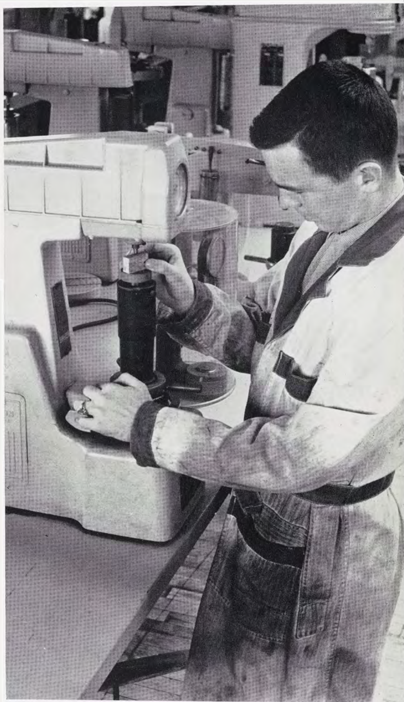
A metallurgical engineering student uses this equipment to test the hardness of different types of metals. Engineering training includes the operation of many types of machinery and motors.
