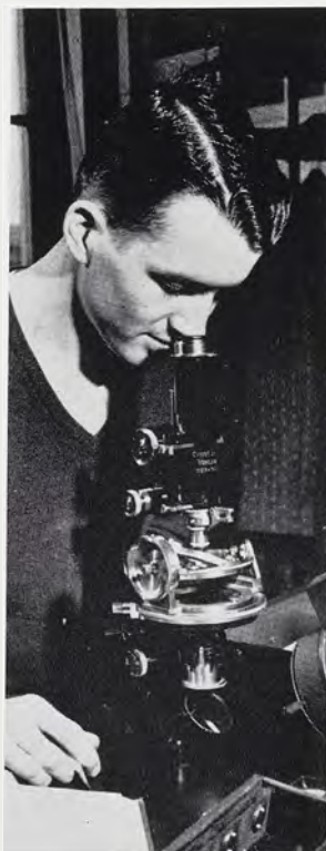
A geology student examines a rock section through a polarizing microscope in a lab.
