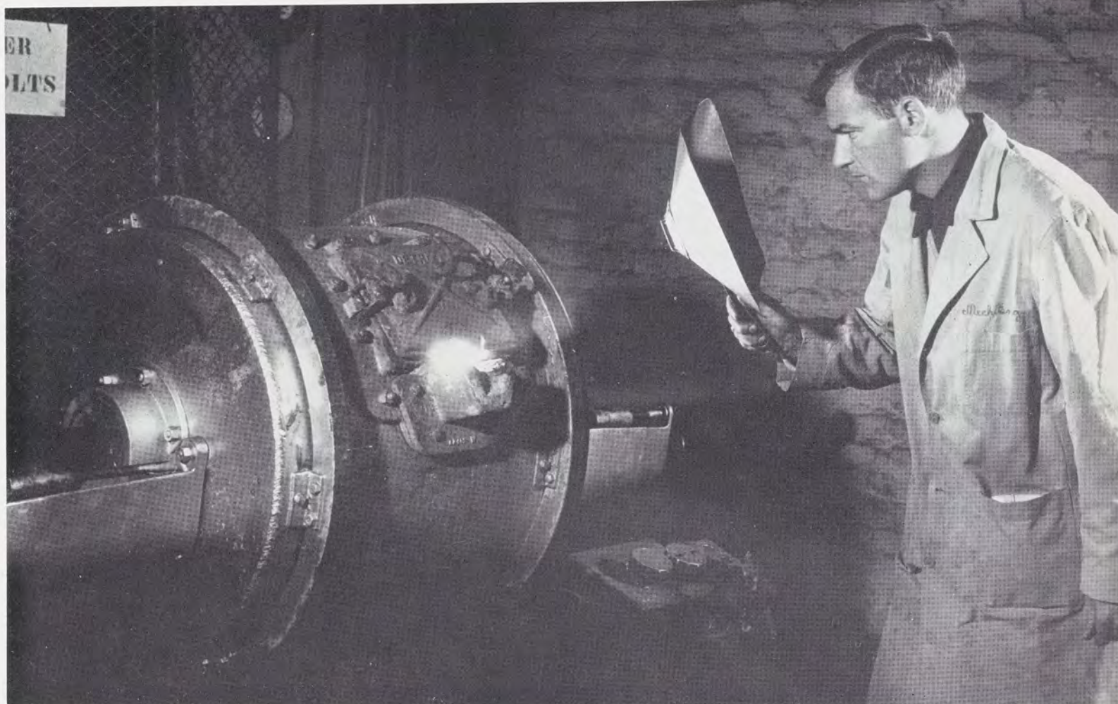
With a protective face shield in front of him, a student checks the temperature of grey iron in an arc furnace melting cast iron.
