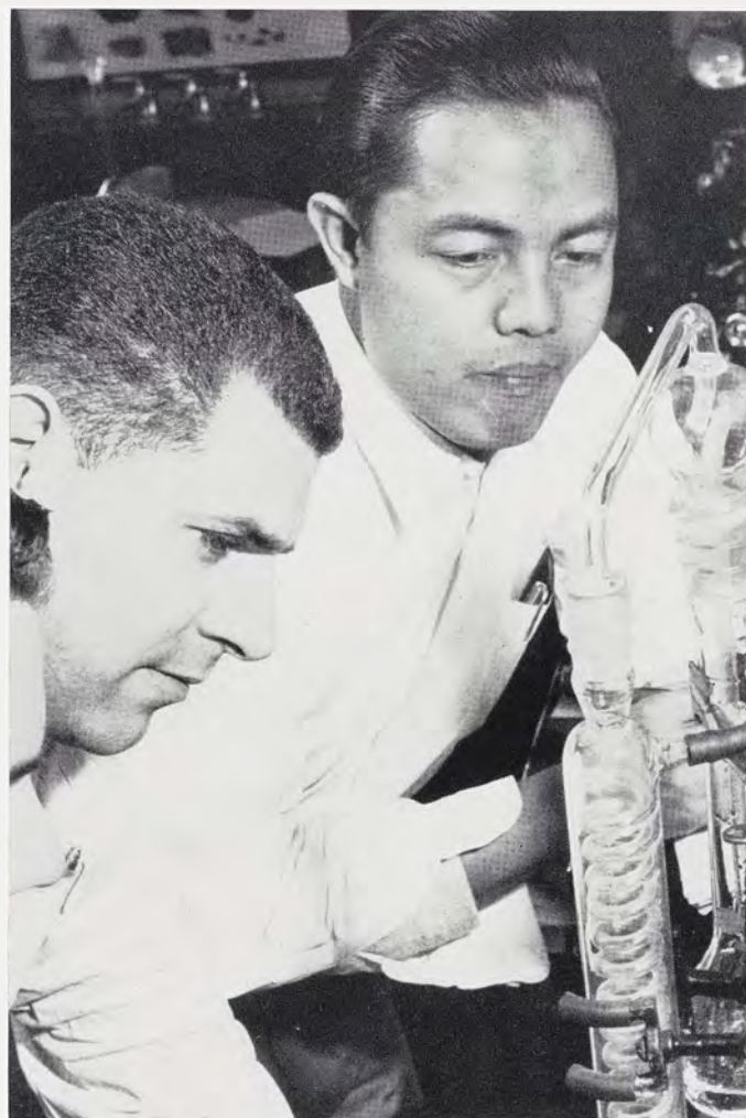
Research and laboratory courses are an important part of graduate training in scientific fields. Two students distill compounds in a Soxhlet extractor.
