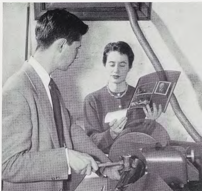
The State News can have pictures ready for the paper within an hour after they are taken because of its Fairchild engraver. Don Hadden attaches the special plastic while feature editor Myra MacPherson scans a finished engraving before it's rushed to press.
