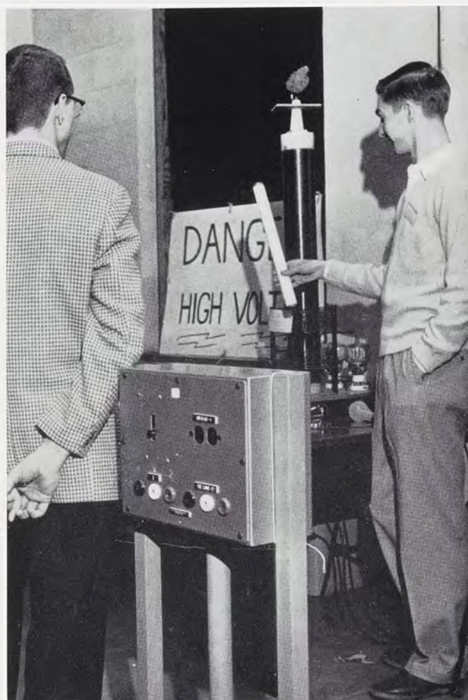
Two electrical engineering students demonstrate a high voltage machine which will light a fluorescent bulb without the use of connections.
