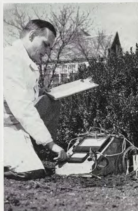
Soil scientist A. Earl Erickson demonstrates the "soil sniffer", a soil analyzer developed by him.
