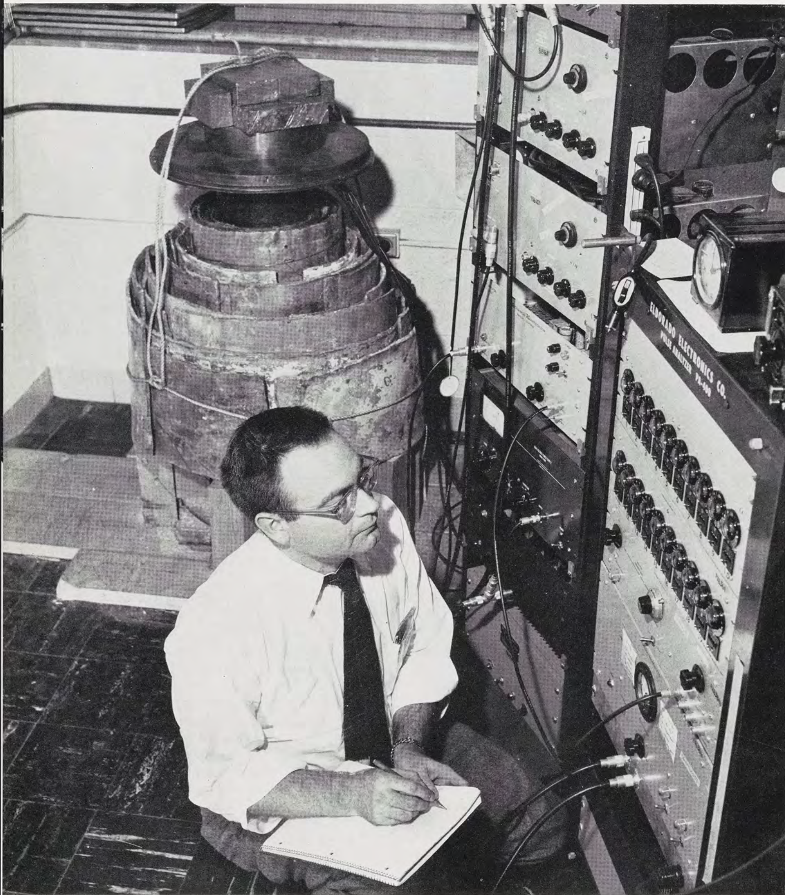
Physicist William H. Kelly reads the meters which record radioactive emissions from a substance contained in the ingenious "sewertron" in the background.
