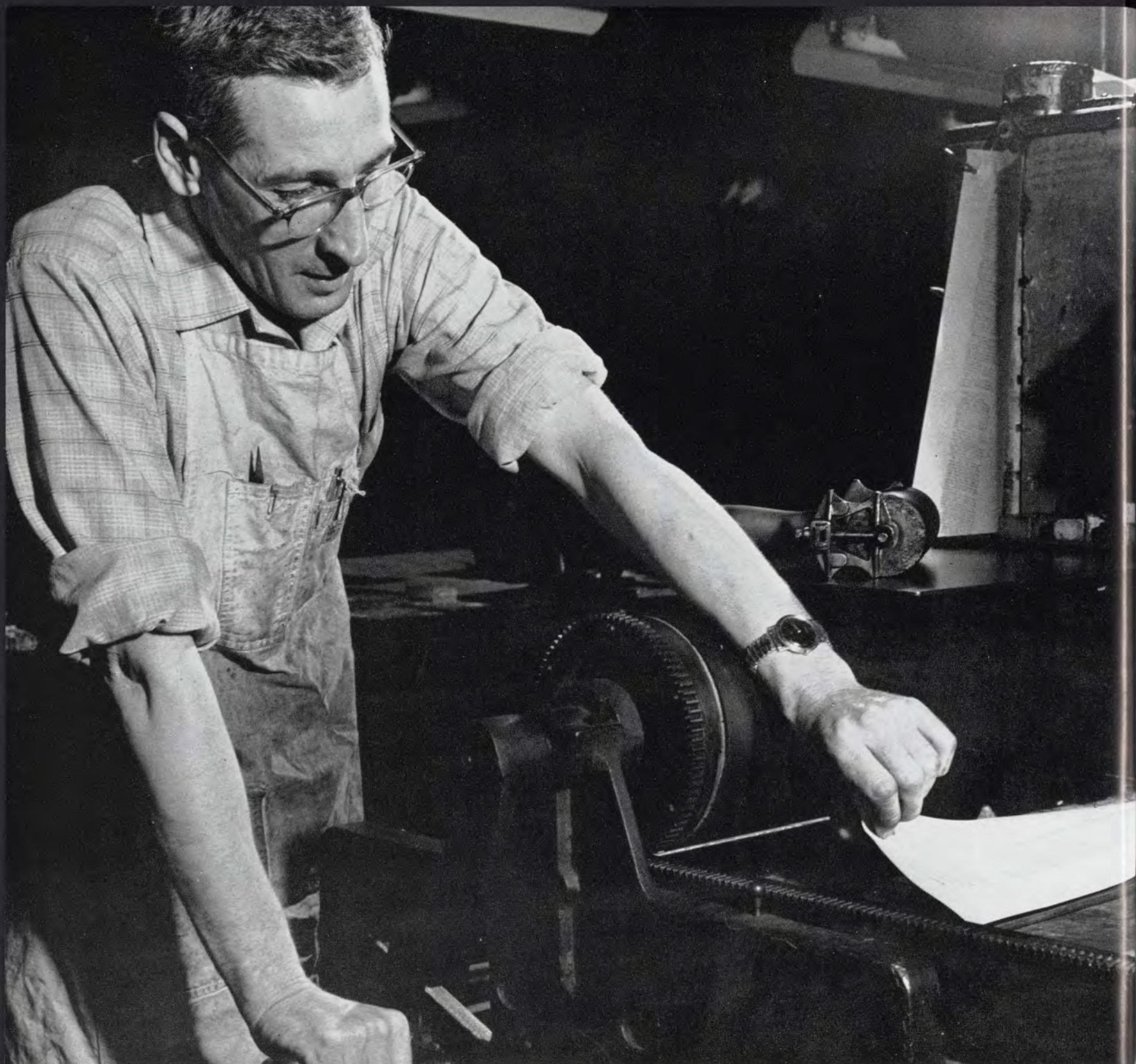
A compositor pulls a galley proof of a column of type at Campus Press where the State News was printed until Spring term.
