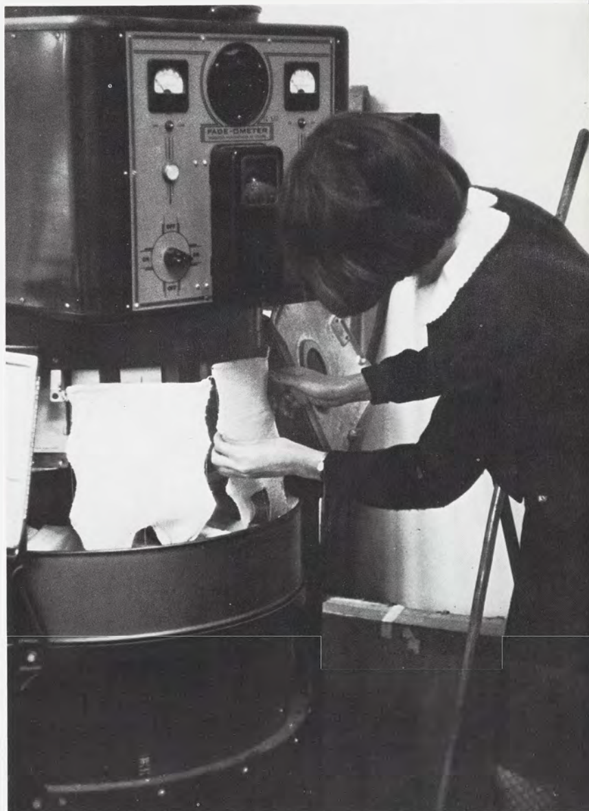
The Fade-O-Meter enables the student to test the colorfastness of fabrics.
