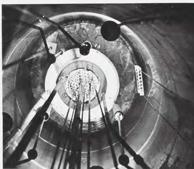
left: Samples irradiated by the products of nuclear fission in the bottom of this well are used by researchers in many departments of the university.
