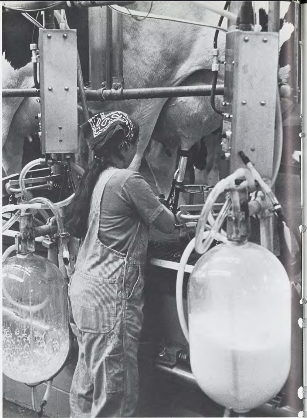
At the dairy barns (below), approximately 110 cows are milked twice a day in the herringbone-model milking parlor (right) which can handle 16 cows at a time.
