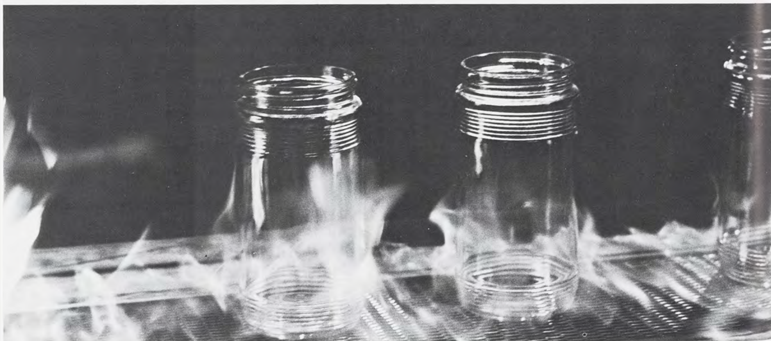
Maggie Walker After being molded, jars are fire blasted as they move along the assembly line.
