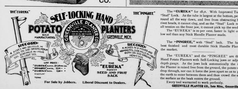
The "EUREKA" for 1898. With Improved Tube and "Stud" Lock. As the tube is largest at the bottom, perfectly round all the way down, and free from obstructing bolt or rivet heads, it cannot clog, and as the "Stud" Lock relieves all tension on the front jaw, it cannot pick up the seed.
