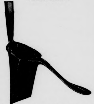
The Eureka Potato Planter, a tube planter with locking jaws and an adjustable depth gauge.
