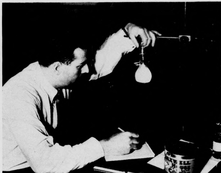
To prove the almost perfect vacuum created in cans of coffee by his newly invented vita-fresh process of packing, T. M. Rector, of the research laboratories of General Foods Corporation, here is shown burning an electric light in a vacuum bulb partially filled with coffee. Any perceptible presence of oxygen would cause the filament in the bulb to burn out instantly.
