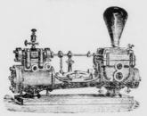
Plain Slide Valve Engines with Throttling Governors.
