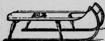
No. 85—Length 30 inches; width 11 inches. Two knees, framed, glued and mortised into runners at two angles with square tenons. Decorated and painted top. Flat shoes. No. 86—Length 33 inches; width 12 inches. Otherwise as above.
