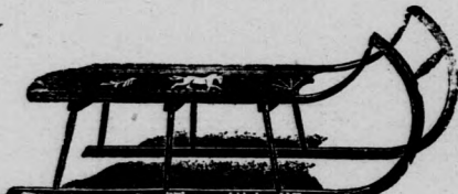
No. 87—Length 36 inches; width 12 inches. Three frame knees mortised into runners, set at two angles in square tenons. Painted and decorated top. Flat shoes. No. 88—Same as No. 87 except with goose necks.
