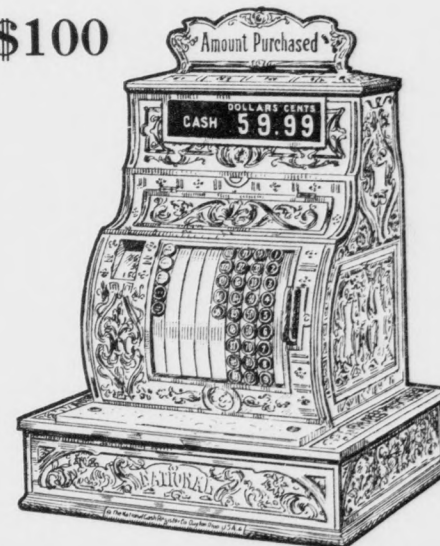
No. 1054 Total Adder, drawer operated, with all latest improvements; prints each sale on a strip of paper 32 Amount Keys Registering from 1c to $59.99, or 5c to $59.95 5 Special Keys
