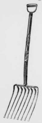
In shoveling potatoes or other vegetables from wagon box or floor with the forks as they have been made, either the load on the fork must be forced up hill sharply, or the head of the fork lowered as the push continues. If the head of the fork is lowered the points will be raised and run into the potatoes. The sharp edge of oval-tined forks will bruise potatoes and beets, and the ordinary points will stick into them.
