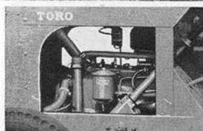
The new Ford Army Scout Car Tractor Engine — Four speed transmission, Clark heavy-duty rear axle, 69 $\frac{1}{2}$  inch wheel-base, 5.50 x 16 front, 7.50 x 18 rear tires.
