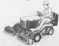
The 2653 features the unique combination of hydraulic reel drive and John Deere 26-inch cutting units.
