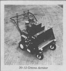
SALSCO products are known for Quality and Performance. No aerators on the market can outperform the FTA-60-24... 128 holes per square foot, 60,000 square feet per hour... or the 30-12... 36 holes per square foot, 13,900 square feet per hour. From self-propelled drop spreaders to powerful truck loaders, every one of SALSCO's twenty products is a rugged, state-of-the-art piece of equipment.
